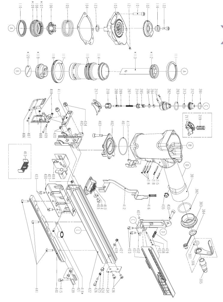
C-W1638P-B1 16 Ga. 15/16" Crown Stapler Exploded View Diagram-Dec. 2017
